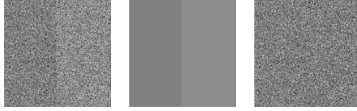
Fig. 4. From left to right: Given a synthetic noisy image I = S + N , the clean image contains one weak step edge, while the pure noise image N is composed of pixels whose intensity values are distributed normally.
